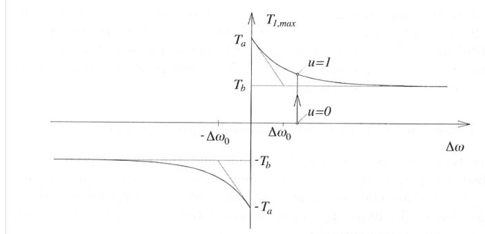
Approximation of the maximum torque in a friction clutch
