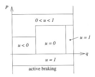
Determine control output as function of some selected state variables: vehicle speed, engine speed, state of charge, power demand, motor speed, temperature, vehicle acceleration, torque demand.
